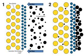
1. Contamination carried on the air flow varies greatly in size, from large particles (like sand) to sub-micronic particles. As the air flow penetrates the filter media, the particles will be arrested by the nanofiber coating on the surface of the media.
