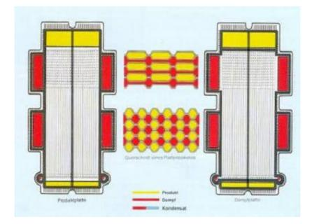
The SIGMA**STAR**<sup>®</sup>-90V and the SIGMA**STAR**<sup>®</sup>-45V can be combined in many different ways to increase the flexibility of our systems, especially for small duties. As the dimensions of both plates are identical, the same frame supports can be used. Expansions and modifications involving both plate types are possible at any time.
