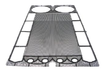
Each of these pressed plates is approximately 0.9 m wide, 1.8 m high with longitudinal, sinus form corrugations, which extend over the full width of the plate. The flow passages on the plates are sealed by gaskets held in place by adhesive. This construction has several technical advantages.
